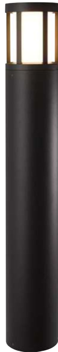
LB-123 Watt: 18W Dimension(mm): 145x900 LED chip: SMD-EVERLIGHT Material: ALUMINIUM+PC Body color: DARK GREY CCT: 3000K CRI: >80 Beam Angle: 360° Luminous Flux: 1062LM IP: IP54
