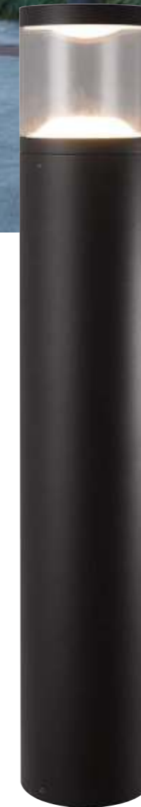
LB-125 Watt: 9W Dimension(mm): 147x900 LED chip: SMD-EVERLIGHT Material: ALUMINIUM+PC Body color: DARK GREY CCT: 3000K CRI: >80 Beam Angle: 360° Luminous Flux: 814LM IP: IP54
