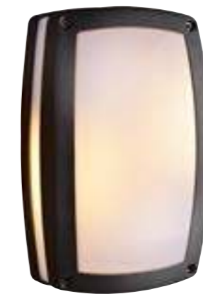
LWL-013 Watt: 18w Dimension(mm): 180x290x87 LED: E27 HOLDER Material: Die-cast Aluminium Body color: Black CRI: T IP: IP44
